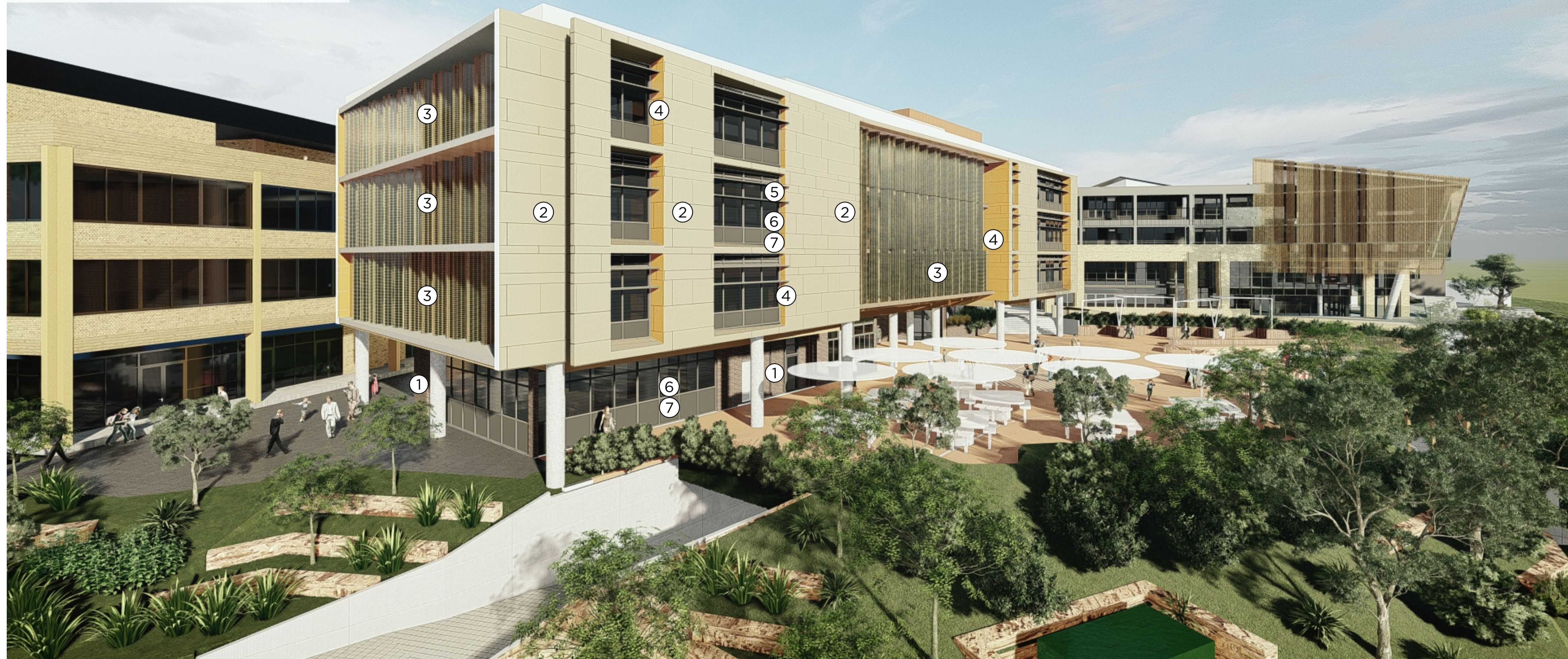
5. Prefinished dark tone metal horizontal sun shades
